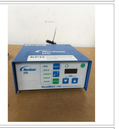
These controllers insure the main control of the deposit size.
